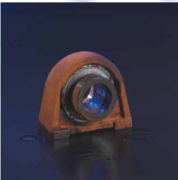
Housing unit affected by corrosion
