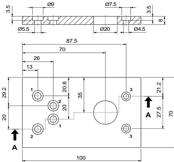
The plate must be fixed on the head using holes "1" and "3" or "2" and "3" depending on side of mounting (left or right). To fix the plate it is necessary to remove the fixing screws on the head in correspondance of the holes "1" or "2".
