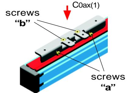
**XSP37** sliders can be used in either "C0ax(1)" or "C0ax(2)" directions (see explanation on previous page). To set the slider preload inside of the rail profile or to adjust the preferential load direction, follow the instructions listed below.
