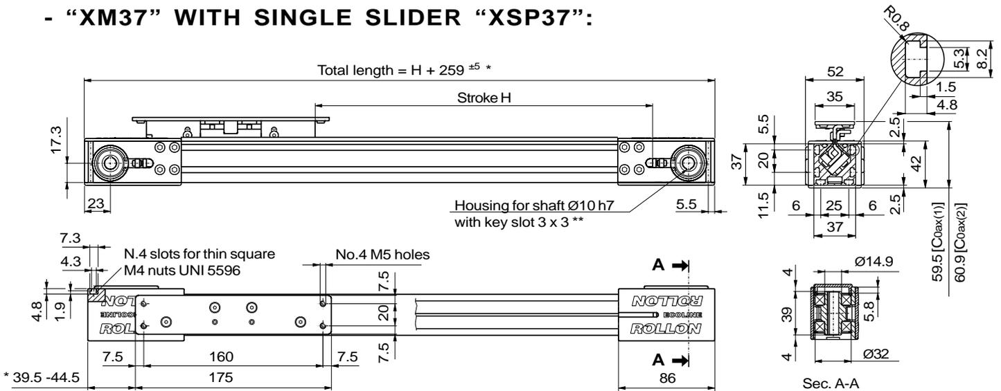
\* Variable dimension according to the head's position after belt tensioning operation.
