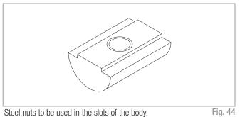
Steel nuts to be used in the slots of the body.
