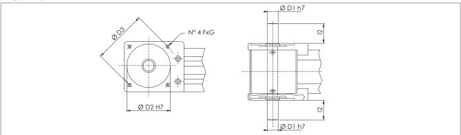
Position of the simple shaft can be to the left or right of the drive head.
