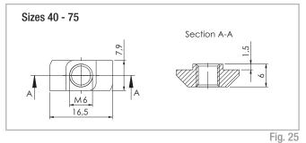
The maximum tightening torque is 10 Nm.
