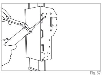
Insert the tip of the grease gun in the specific grease blocks.
