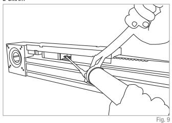
Quantity of lubricant necessary for re-lubrication for each block:
