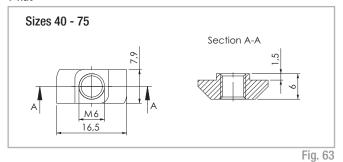
The maximum tightening torque is 10 Nm.
