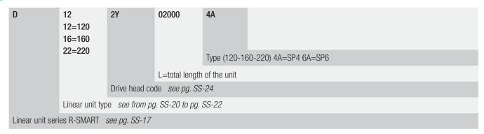
In order to create identification codes for Actuator Line, you can visit: http://configureactuator.rollon.com
