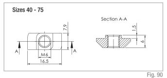
The maximum tightening torque is 10 Nm.
