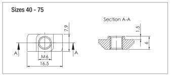
The maximum tightening torque is 10 Nm.
