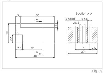
Fixing clamp for simple mounting of a linear axis on a mounting surface or for connecting two units with or without a connection plate (see pg. US-68).
