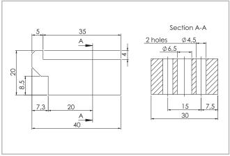
Fixing clamp for simple mounting of a linear axis on a mounting surface or for connecting two units with or without a connection plate (see pg. US-68).
