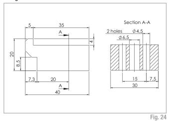
Fixing clamp (for all sizes except A100) for simple mounting of a linear axis on a mounting surface or for connecting two units with or without a connection plate (see pg. US-68).
